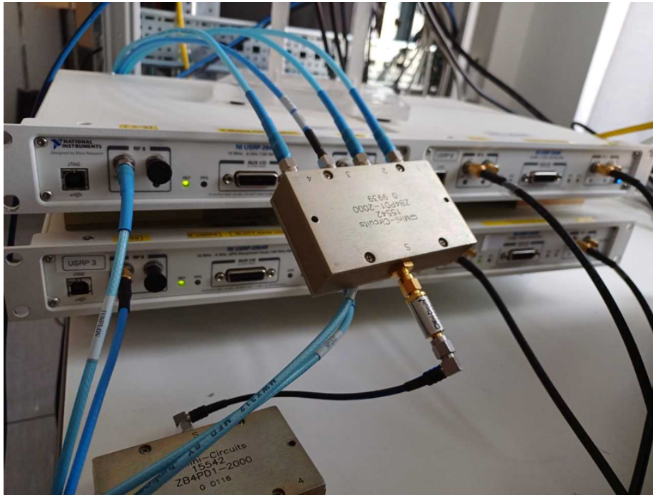
Figure 10-3: Flexible transceiver laboratory setup with combiner.
